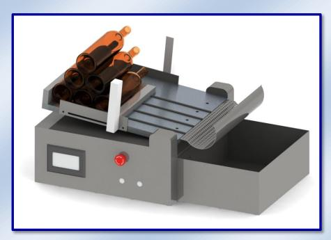
Bottle Tilt Tester is a standard equipment to measure and evaluate the bottles resistance to tilt Mainly used by glass, beverages, pharmaceutical, cosmetic industries.
