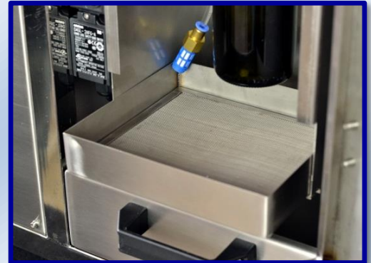
Trash bin design with silencing sifter
