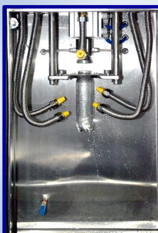
PABT with hot water spraying system (Optional)
