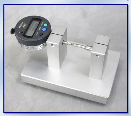
PTG -1 Plate Thickness Gauge is for quick checking of the thickness of plates.
