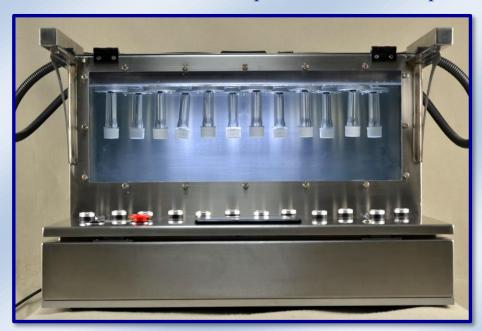
The SSA-PLC-12 Secure Seal Analyzer (12 Positions) is a special instrument developed by AT2E for control of the secure seal performance of caps on preforms.
