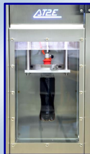
Automated piercing and testing with AT2E patent needle
