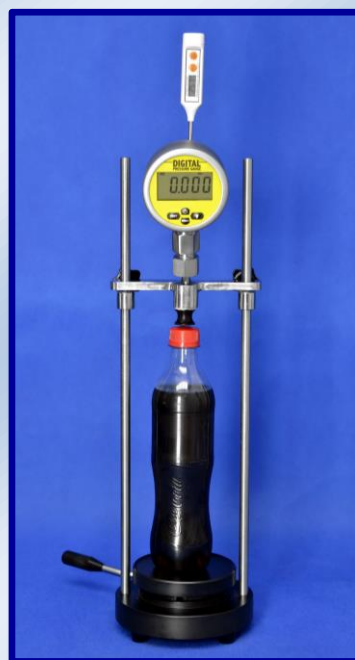
CO 2 EASY-D with digital pressure indicator
