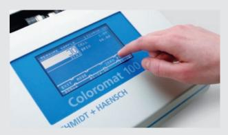
The **touch screen** is used for soft key functions and alphanumerical inputs which allows easy handling for example batch name, user etc.. The wavelengths are selected via the touch screen. **Three wavelengths** are pre-installed as standards, optional the Coloromat 100 can be equipped with **six further** customized **wavelengths**. This opens a wide range of applications.
