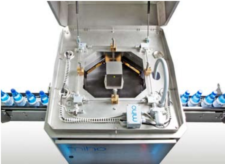
Height adjustable camera and lighting system
