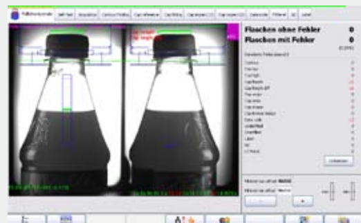
Cap Inspection: tilted cap
