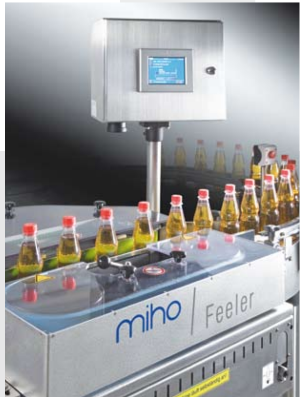
Sealing inspection using a sensor wheel (subject to patent). See illustration of sensor wheel on page 5.
