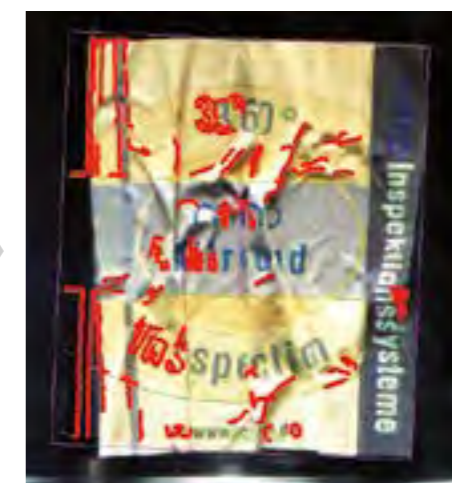
Detection of the „crease“ fault on the basis of the miho image-processing platform miho VIDIOS®
