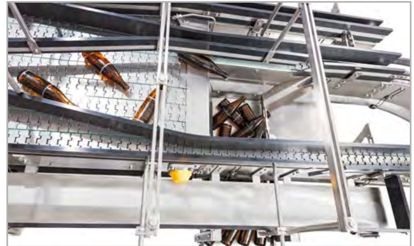
miho Conveyance, individual special solution for collecting lying bottles in hard to reach places
