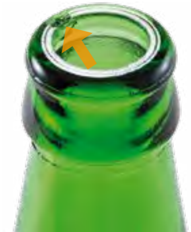
Glass: chip on the sealing surface
