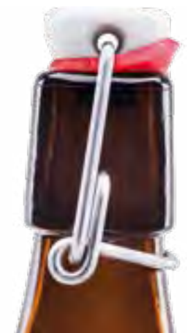
Distorted rubber seal
