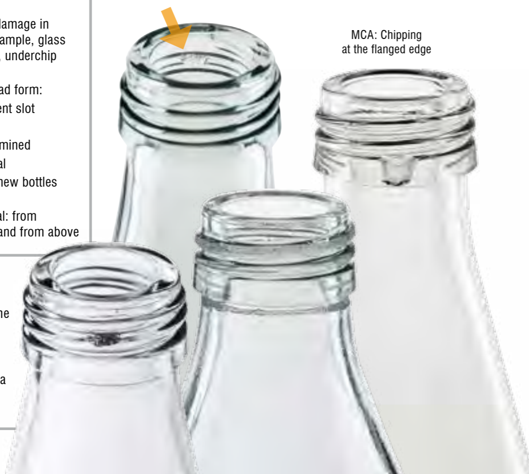
MCA: Dirt in the threaded area
