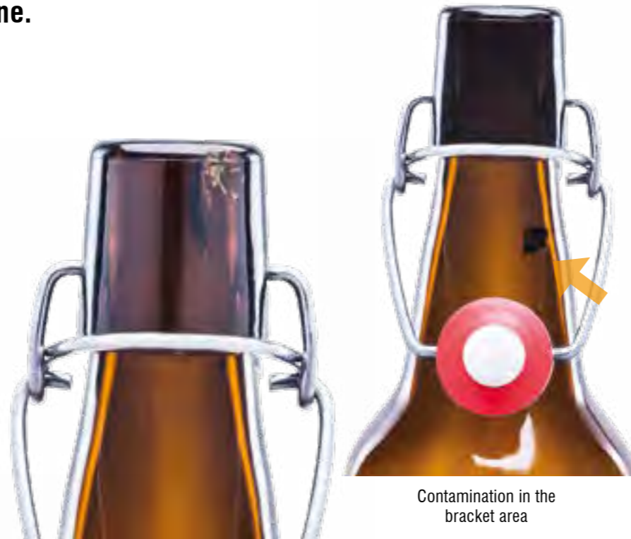
Swing top bottle with vertical split in the finish area
