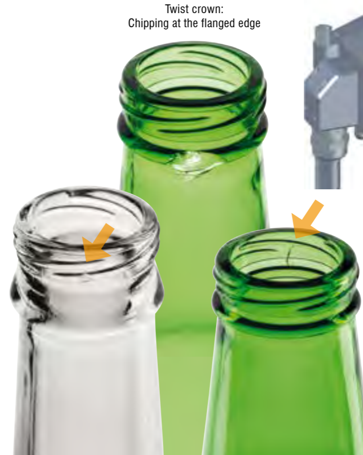
Twist-Crown: Thread defect
