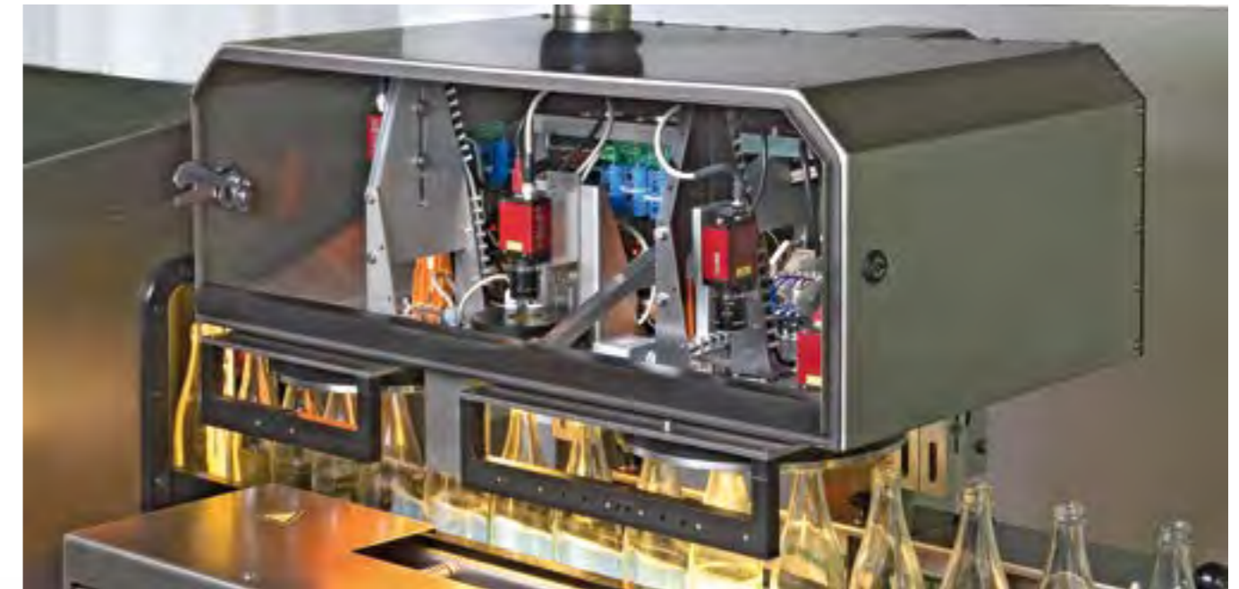
Inspection head of the basic machine, opened
