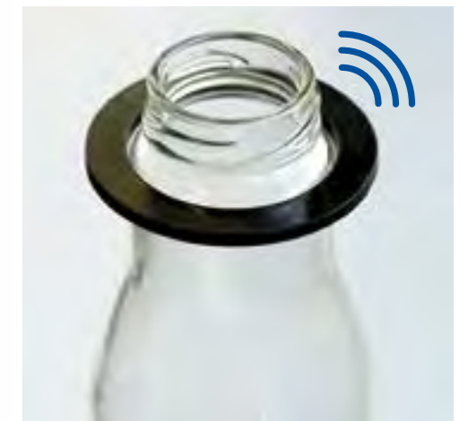
Test bottle with transponder ring attached
