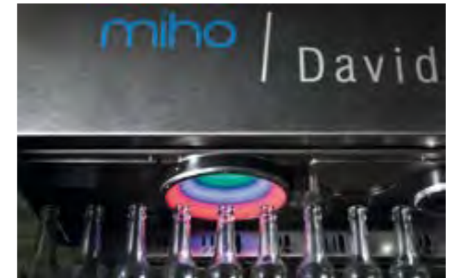
The LED colour lighting ring in operation
