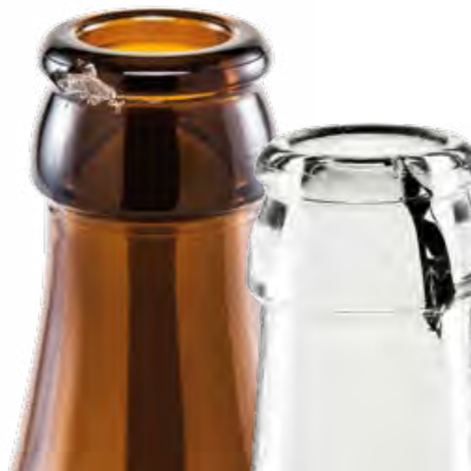
Crown corks: Underchip defect
