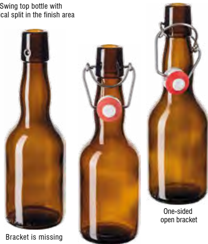
Bracket mounted the wrong way round
