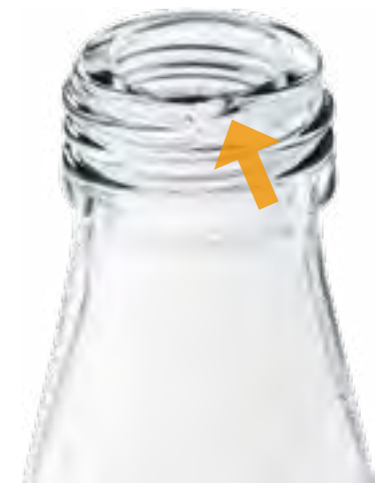
Glass: chip on the sealing surface
