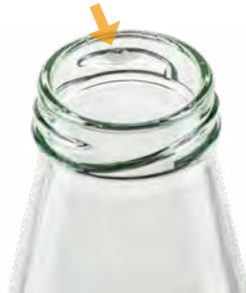
Twist-Off: Thread defect
