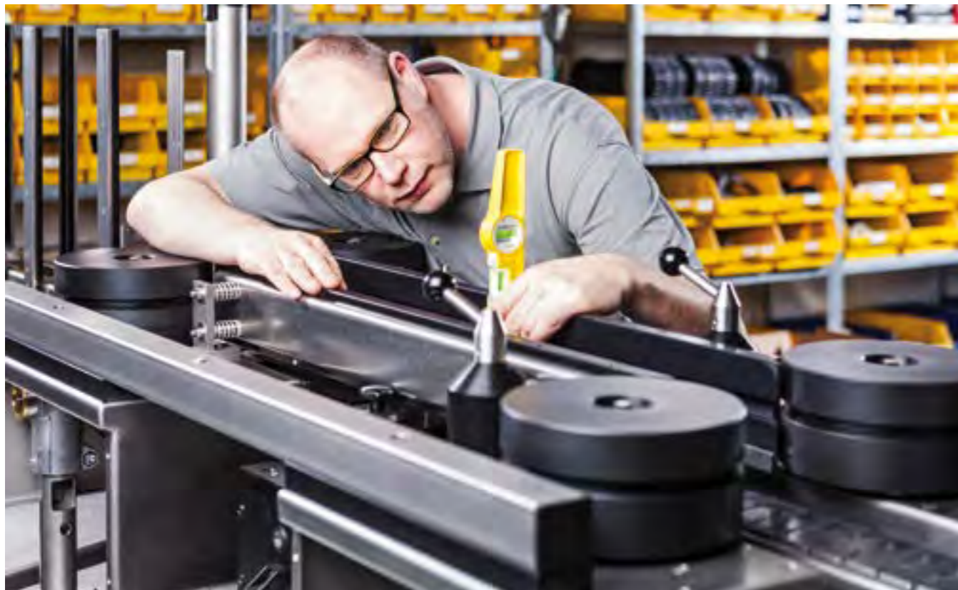
Mechanical installation of the miho David 2 basic machine
