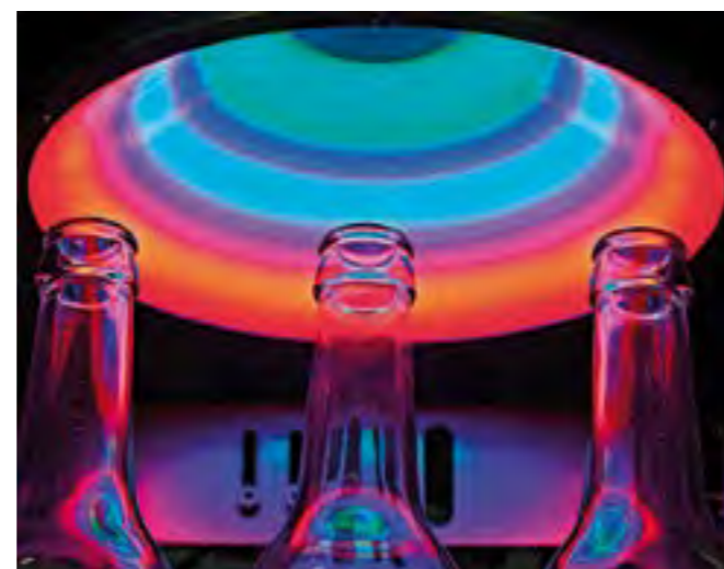
Sealing surface inspection with RGB lighting
