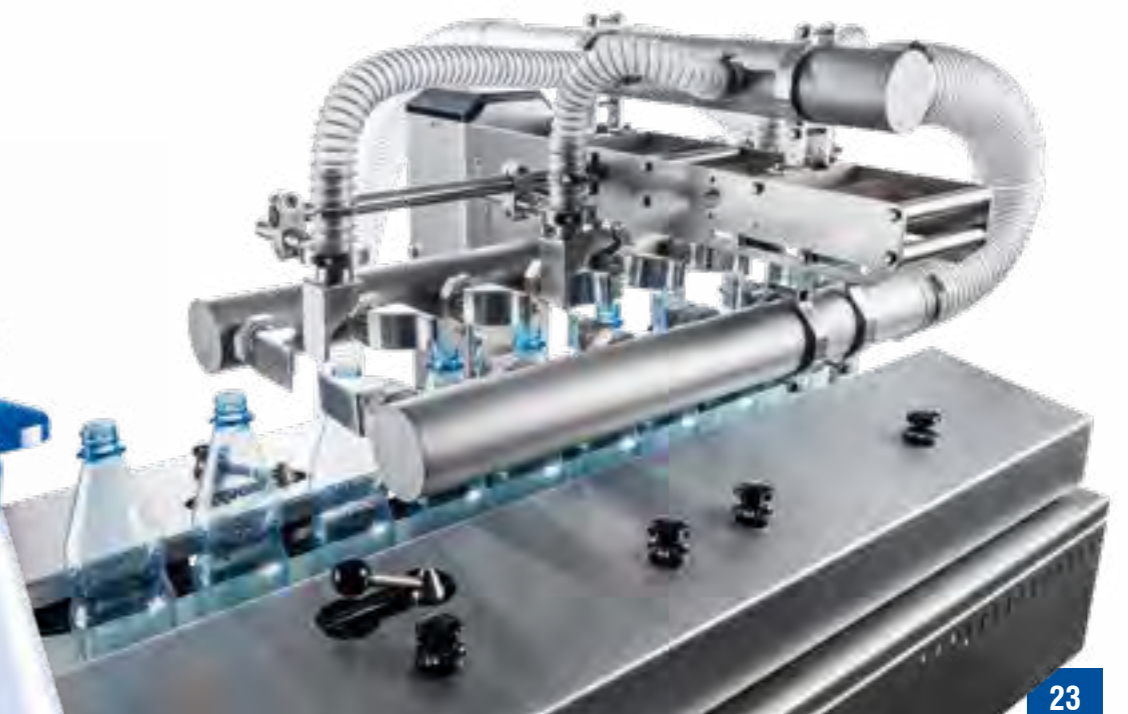
For blowing off PET bottles: miho Bottle Dryer
