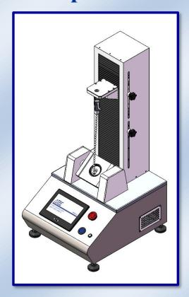
AT2E PATT-1 Pop and Tear Tester provides a complete solution for easy open ends inspection. It is able to measure the pop and tear force of different types of easy open end with different test modes. It has been widely used in can, food and beverage industry.
