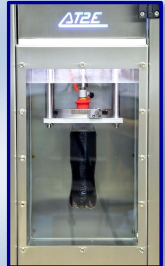
Automated piercing and testing with AT2E patent needle
