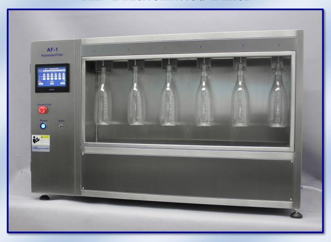
AT2E's AF-1 Automated Filler is designed as a quick water filling device of bottles. It's mainly used to improve the efficiency for some tests which require a filled bottle, such as stress crack test, secure seal test, burst test and so on... It can fill 6 bottles in 1 time at predefined volume with high accuracy.
