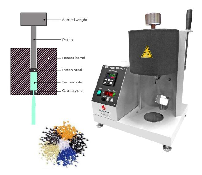
The fluidity index is a basic rheological test that is performed on a polymer to determine its fluidity. It is measured in g/10min. It is defined as the amount of material (measured in grams) that flows through the hole of a capillary die in 10 minutes, maintaining constant pressure and standard temperature.
