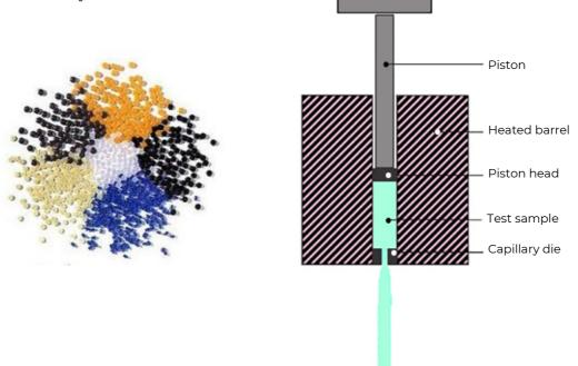
This index is of vital importance for those who make injection molding, extrusion, broken molding or any other process that involves the manufacture of a thermoplastic part.
