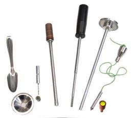
**Spatula** and pellet feeding **funnel**, Tungsten Carbide Ø 2,095 mm **capillary die**, Capillary die **cleaning tool**, **Piston**, Cylinder **cleaning tool**, **Extrusion tool**, **Plumb line**, **Bubble level** and **Tweezers**.
