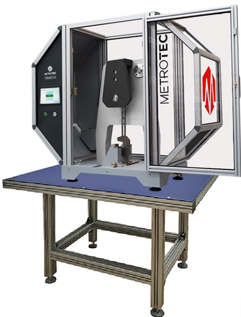
PIT-25 Impact Pendulum + Support Table (compliance standards >15 Joules)
