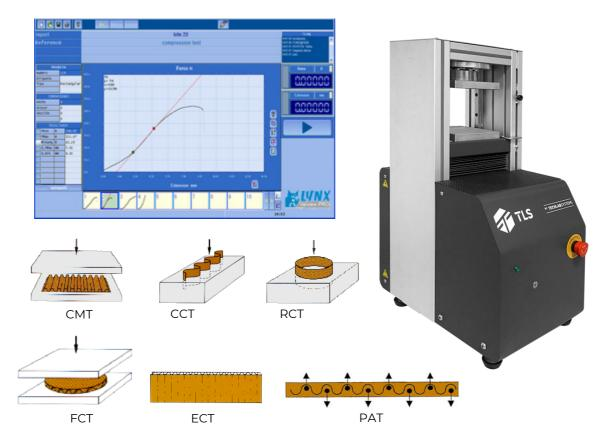
The Testing Software allows to perform Compression tests on standard samples of corrugated paper and cardboard such as: CMT - RCT - CCT - ECT - FCT - PAT
