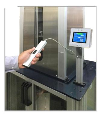
NOTE: We can build the impact resistance test equipment according to ASTM D 2444 with drop height of the striker impact of 3 m (please consult).
