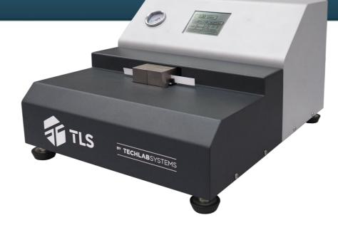
This testing equipment is used to measure the compressive strength of paper and cardboard samples by the SCT method (0.7mm short distance compression between jaws). The test is performed using a 15 mm wide paper or cardboard specimen and it is compressed until failure occurs.
