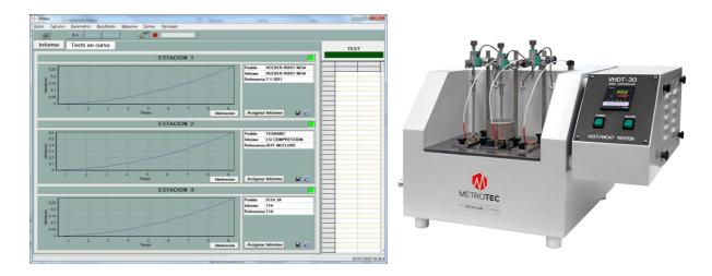
The Testing Software allows testing and determining the VICAT softening point and HDT Flex temperature on samples of thermoplastic materials.
