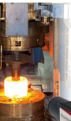
The **view finder** provides upright imagery so that the target under measurement can be viewed visually. A circular reticle shows the measuring spot. Recommended for glowing measurement objects, as a red laser is difficult to detect. For devices with measuring range above 1800°C, the eyepiece can be darkened for eye protection.
