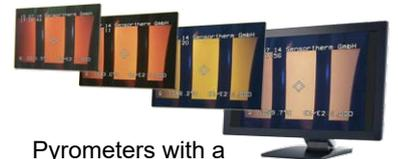
Pyrometers with a **color camera module** provide a composite video output that can be connected to a video monitor or PC with a converter. The pyrometer is aligned via a circular reticle on the TV screen and is recommended for remote observation of glowing hot targets or viewing down sight tubes. The camera provides automatic, highly dynamic adjustment of the picture brightness.
