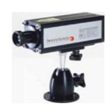
For none contact temperature measurement of thin polyester films and all kind of fluorocarbon-plastics the narrow band model  $Metis\ MY80$  was developed. Further more it is best choice to measure thin glass surfaces in furnaces because glass is neither transparent nor reflective at 8,05  $\mu$ m. It meets therefore the so called black body conditions of an ideal radiator.
