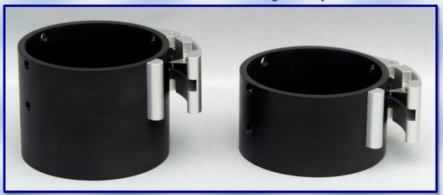
The "SSC-1" Simple Section Cutter is a simple tool for section cutting of a plastic bottle. It provides a fast and repeatable cutting process for section weight control. Operator just needs to inset the bottle to the cutter, press the lever to let knife piece into the cut position and twist the bottle. Then the demanded section can be obtained.
