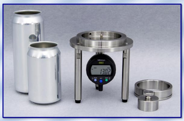
CDDG-1 Can Dome Depth Gauge is specifically designed for measuring the dome depth of beverage can. With the quick changing spacers, it is easily compatible with cans of different diameters.
