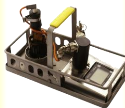
Pasteurization Monitor - RPU
